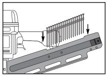
Figure 2. Loading the nailer.
